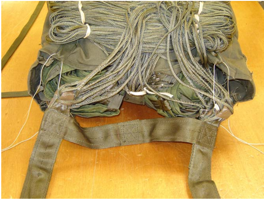
Figure 26. Riser Securing Ties Positioned.
